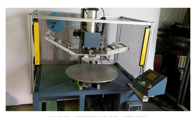
MODEL PT – 3, THREE TON HEAT TRANSFER PRESS 30" ROTARY TABLE, 3" STROKE ADJ. HEIGTH RAM SAFETY CURTAIN, 480V, OVERALL DIM 64" X 48" X 86" CAGED REMANUFACTURED BY HASTINGS ADS
