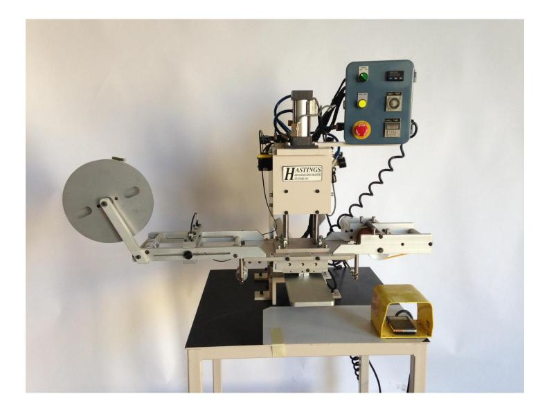
MODEL US 1, HALF TON HEAT TRANSFER PRESS. 5" X 5" HEATED HEAD ON A MACHINE BASE CURRENTLY SET UP WITH FOOT CONTROL & SAFETY BAR AROUND PINCH POINT TYPICALLY USED IN THE TEXTILE INDUSTRY, REMANUFACTURED BY HASTINGS ADS.
